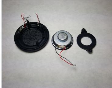
After the speaker is detached, remove the two 8.5mm screws that hold the speaker to the front panel with a Phillips #1 screwdriver.
