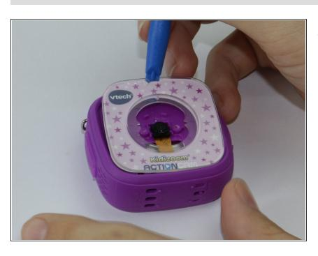
Pry off the transparent plating and paper design using a plastic opening tool.
