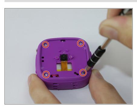
Unscrew the (4) 2.5mm Phillips head screws from the third layer of plating using a #0 screwdriver.
