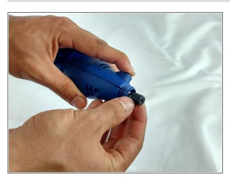
While pressing the spindle lock button, unscrew the collet nut and remove it along with the brass collet.
