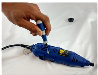
Unscrew the six 8mm PH2 screws.
