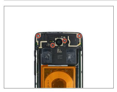
Remove the four Torx T5 screws securing the midframe plate.
