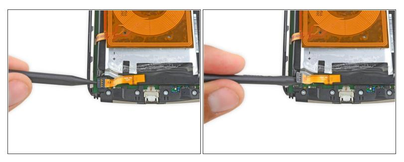
• Use the point of a spudger to pop up the battery connector.
