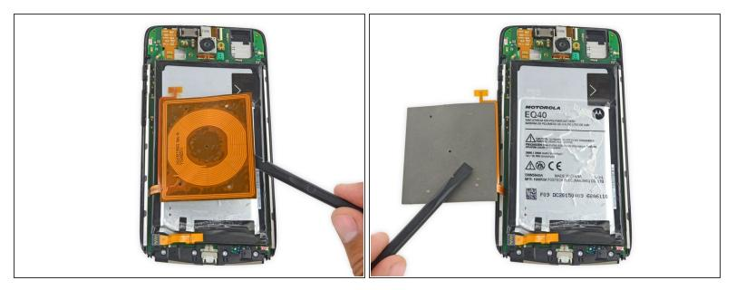
• Fold the wireless charging coil away from the battery.
