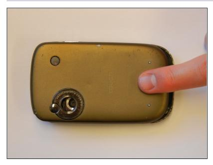
• Using your finger, remove the back panel by sliding it up.
