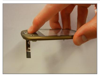
Remove the small circuit board by gently pushing on the center button on the front of the phone.
