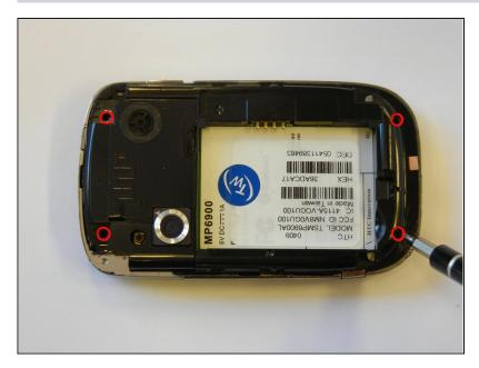
Remove the four screws in the corners of the phone using the T5 Torx screwdriver.
