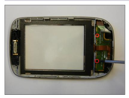
Remove the two screws from the back of the front panel using the Phillips #00 screwdriver.
