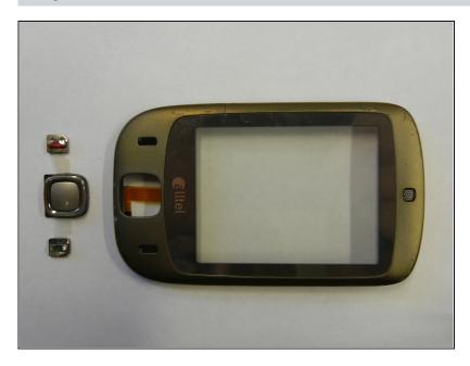
Remove the buttons by pushing on them from the front side of the phone.
