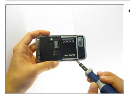
• Using the Phillips #00 screwdriver, remove the phone's battery.
