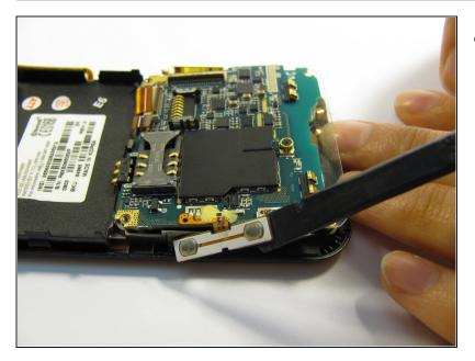
• Peel the button sensor on the side of the motherboard off of the case.
