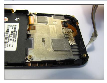
• Peel up the black tape on the bottom of the back case.
