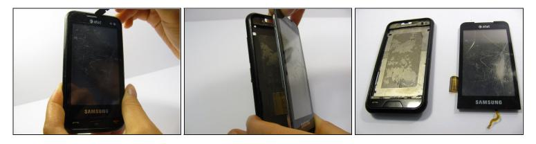
• Use a small tool to pry the digitizer and screen (together) from the frame of the phone. This may take some time and careful work because it is glued down to the frame.
