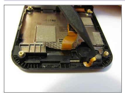
• Pop the microphone up and out of its small housing.
