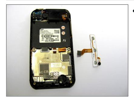
• The front button board should slide out. At this time you can replace the button/microphone component.
