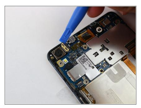
Loosen the camera from the glue using the small blue plastic opening tool.
