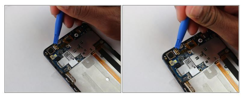
• Disconnect the contact patch using the small blue plastic opening tool.
