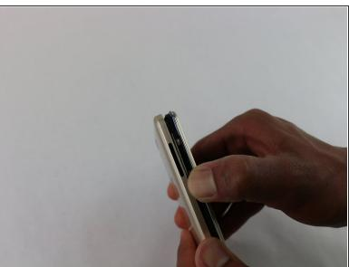
Take the blue plastic opening tool and insert it in-between the back of the phone and the chrome trim. Go all the way around the device slowly to take the back cover off.
