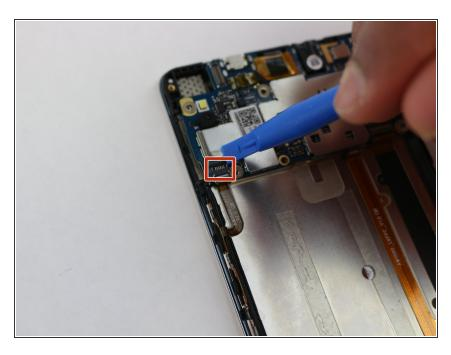
Lift the black tab on the zero insert force connector on the lower left side of the motherboard using a small blue plastic opening tool.
