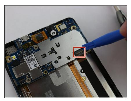
Lift the black tab on the zero insert force connector on the lower right side of the motherboard using a small blue plastic opening tool.
