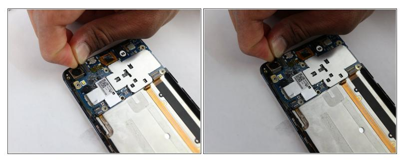
After loosening the glue from the bottom of the camera, lift the camera out of the phone.
