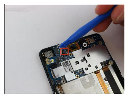
Lift the black tab on the zero insert force connector on the top left side of the motherboard using a small blue plastic opening tool.
