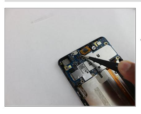
Use a fine nose pair of tweezers to pull the ribbon cable from the zero insert force connector with little force to remove the contact connecter from the motherboard.
