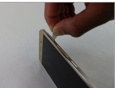
Flip your device to the right side facing up and use the SIM card eject tool to remove the SIM card by pushing the tool in the hole. You will feel a button click and the tray should slide out 2mm. You will then use your fingers to pull the tray out.
