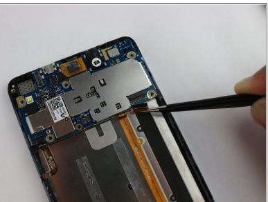
• Use a fine nose pair of tweezers to pull the ribbon cable from the zero insert force connector with little force to remove the contact connecter from the motherboard.
