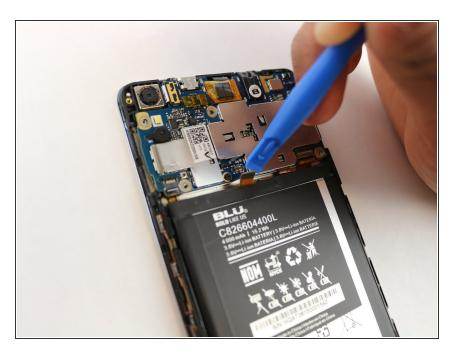
Use the small blue plastic opening tool to lift the contact attached to the battery from the motherboard of the phone.
