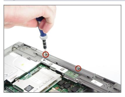
• Remove two screws (5.8mm)
