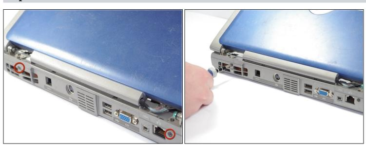
• Using a Phillips screwdriver remove the two screws (5.8mm) located at the rear of the laptop.
