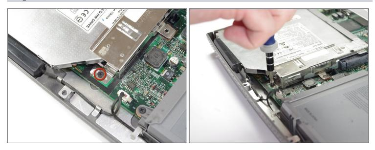
• Remove CD drive plating screw (5.8mm)
