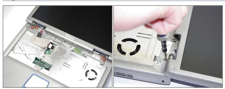
• Using a Phillips screwdriver remove the four screws (5.8 mm) located at hinges of the screen.
