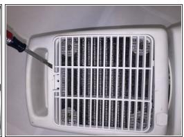
As seen in the pictures, set the screwdriver on the edge of the cover and pry it out.
