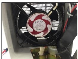
• Unscrew the four screws located in the rear of the device. Remove the fan.
