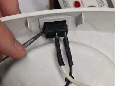
Apply pressure onto the sides of the switch while pushing it outwards.
