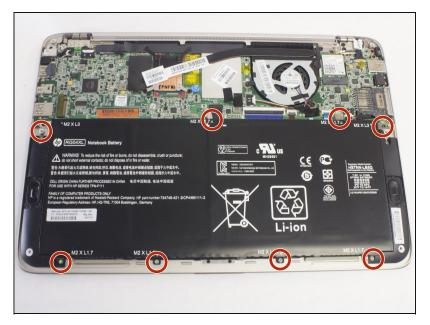
Remove the six 2.0mm silver screws and the two 3.2 mm black screws using the PH00 Phillips Screw Head.
