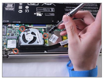
Unscrew three 2.0 mm screws using the Phillips Head #0
