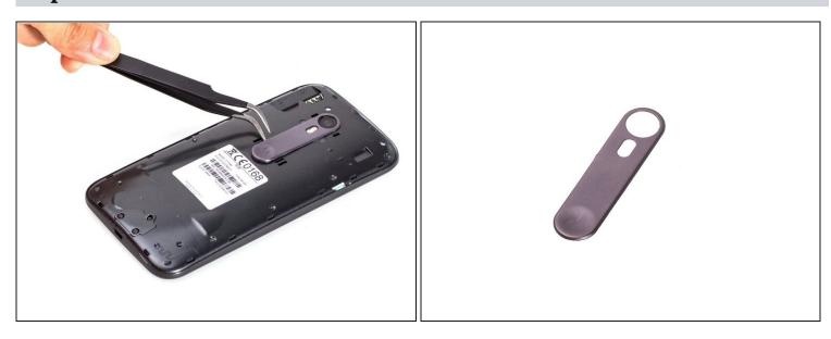
• Remove camera&flashlight metal cover. Use <u>tweezers</u> to cut strong adhesives underneath.
