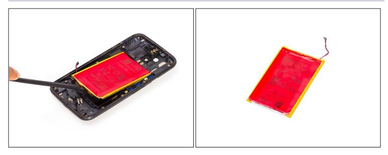
• Use spudger to cut adhesive and pry the battery up.
