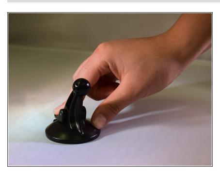
Pull the lever on the back of the GPS mount up and remove it from the surface.
