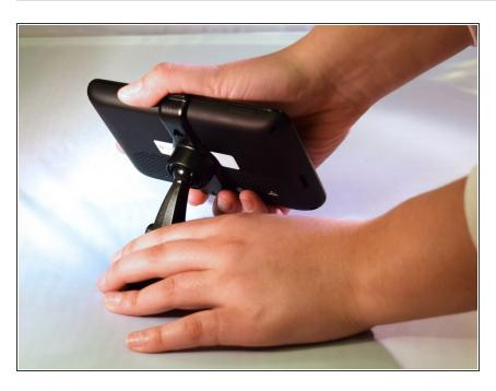
Separate the GPS mounting cradle from the mounting device.
