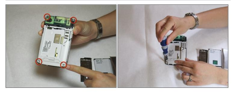
Remove the four screws that secure the front cover to the rest of the phone using a T7 screwdriver.
