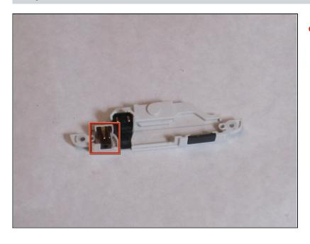
• Remove the headset jack from the housing by pulling it up.
