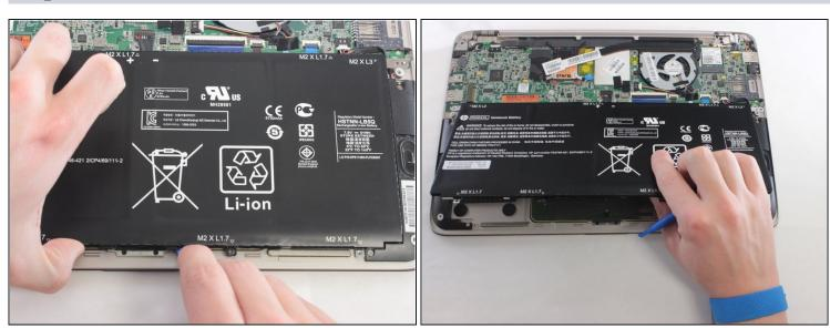
• Gently lift up the battery and remove using the plastic opening tools.
