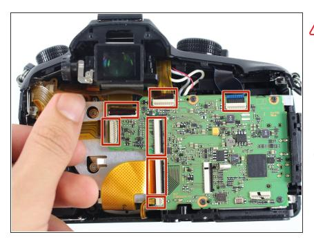
⚠ Do not yank out the electronic ribbons attached to the motherboard, or you may damage them. To properly detach these ZIF connector ribbons, see this technique on disconnecting ZIF connectors.
