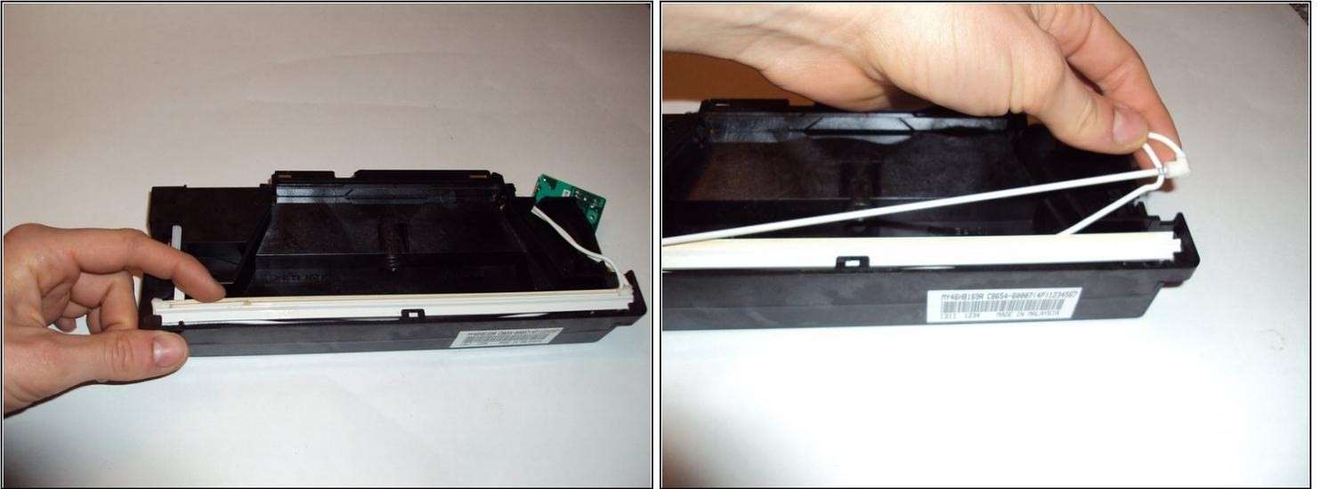
**⚠ Carefully** twist white scanner lamp support out of its carriage and replace it with a new one.
