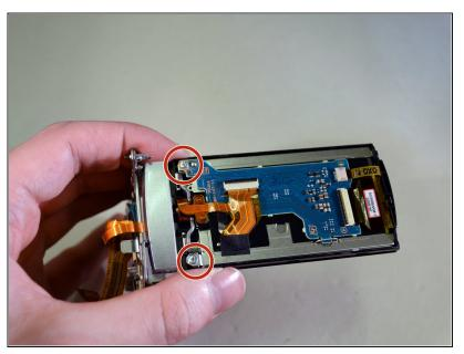
• Remove two silver 3mm Philips screws on left side.
