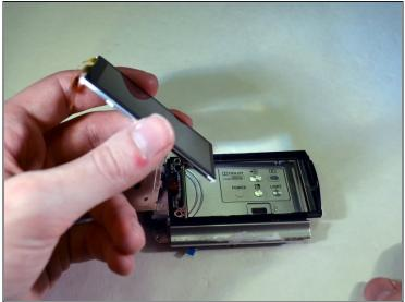
• Lift out the screen by grabbing the ribbon wire and lifting up and out.
