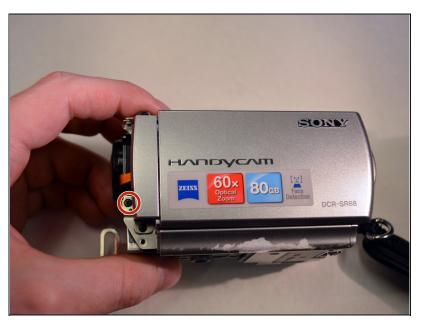
On the left side of the device, remove the middle left 3mm Philips screw.
