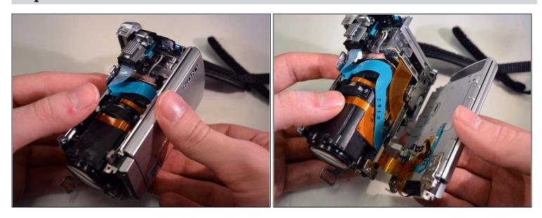
• Carefully pivot the loose left side of the device until the ribbon wires are fully exposed.
