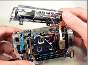
• Remove top of device by lifting up and away.
