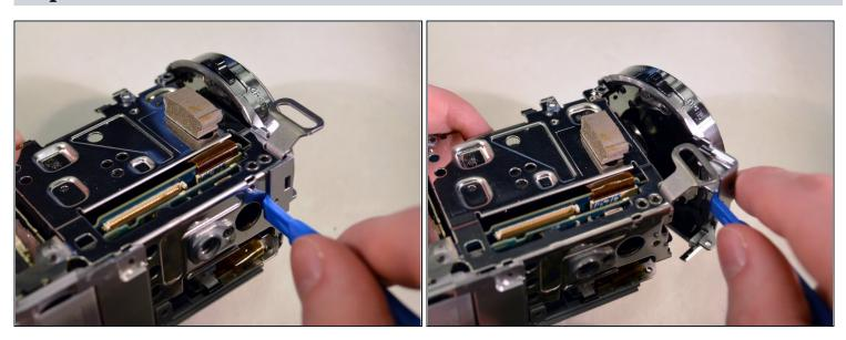
• Use the blue plastic opening tool to pop the shutter assembly off the device.
