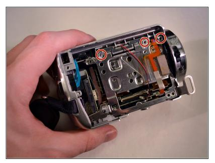
On the right side of the device, remove the top three right 3mm Philips screws.
