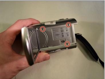
On the left side of the device, remove all visible 3mm Philips screws.
