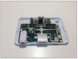
• You can now remove the two screws that secure the weight to the plastic housing.
