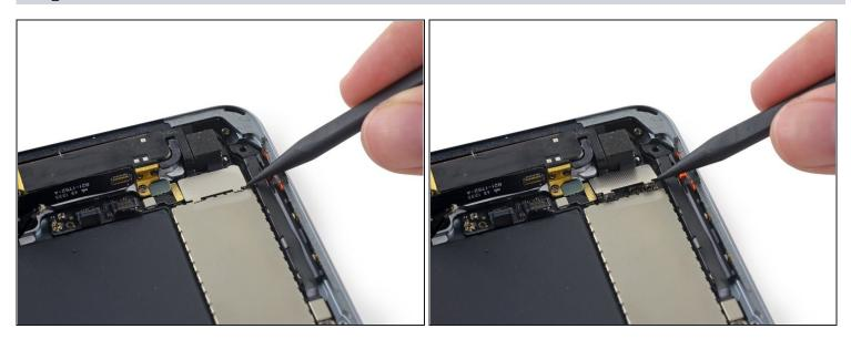
• Use the tip of a spudger to lift the front edge of the bracket.
