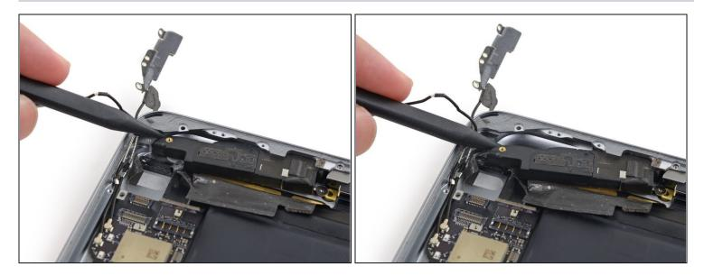
• Insert the tip of a spudger into the gap between the left speaker and the bottom left side of the rear case.
