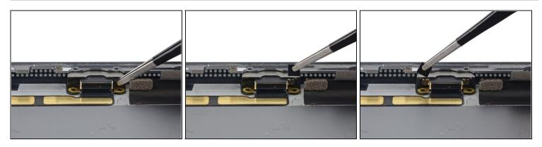
• Use a set of tweezers to remove the small plastic covers on the screws in the Lightning connector housing.
