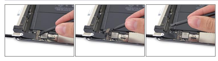
• Use the flat tip of a spudger to gently lift the battery connector up off its socket on the logic board.
