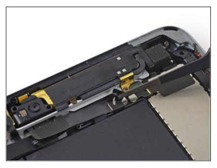
Use a set of tweezers to remove any tape covering the frontfacing camera cable clips.
