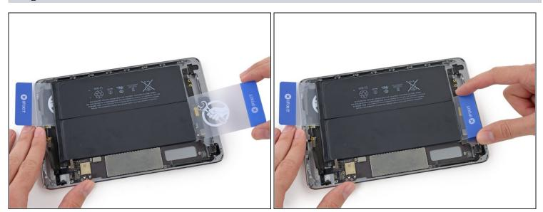
• Insert a second plastic card beneath the battery on the logic board side near the front-facing camera.
