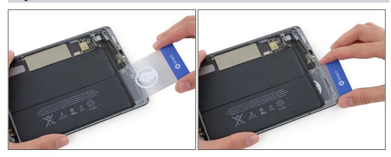
• Remove the plastic card and insert it under the cell nearest the edge of the case.
