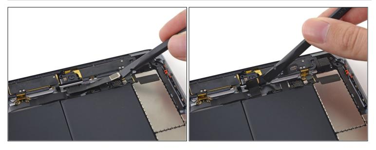
• With the flat end of a spudger, lift the front-facing camera connector straight up off of its socket on the logic board.
