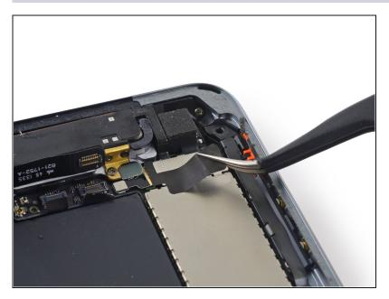
Remove any tape from the rear-facing camera cable bracket.
