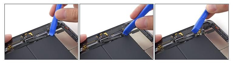
• Use a plastic opening tool to fold the front-facing camera cable clips outward, away from the cable, to free the cable connector.
