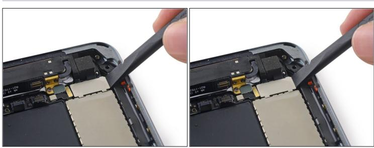
• Use a plastic opening tool to push the rear-facing camera cable bracket to the left.
