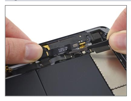
Use a set of tweezers to peel up the small piece of tape covering the headphone jack cable connector.
