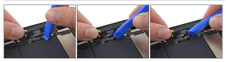
• Use a plastic opening tool to fold the headphone jack cable clips outward, away from the cable, freeing the cable connector.
