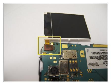
Reattach new screen by connecting the orange ribbon to the computer chip
