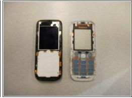
♠ Separate the front case from the back case using the iPod opener
