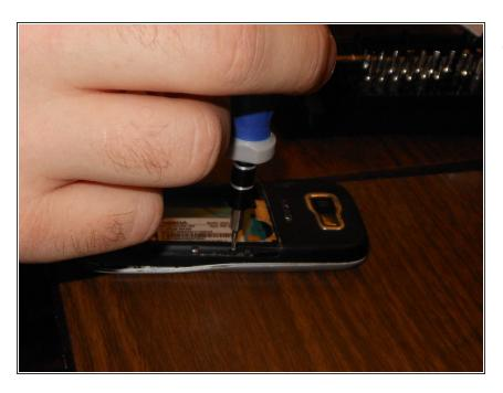
Reassemble screws with microscrewdriver
