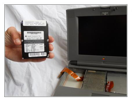
Attach the ribbon cable to the new hard drive and follow steps 1-3, in reverse, to complete the installation.
