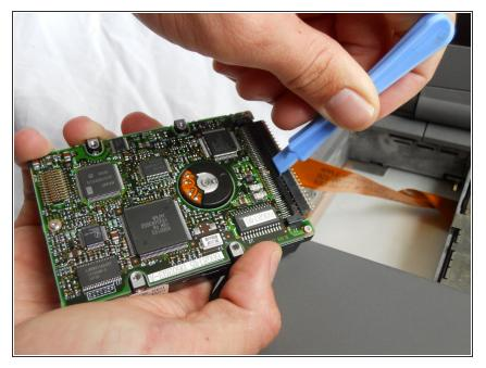
• You can use a spudger (tool shown in photo) to remove the ribbon cable from the hard drive.
