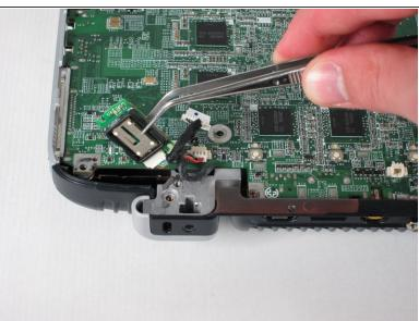
Using tweezers, pull up on the Bluetooth module to remove it.
