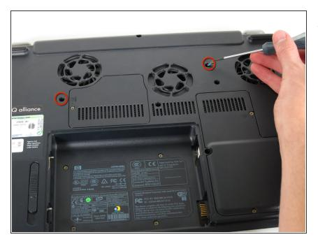
Remove the two 8mm Philips screws marked "K" on the bottom of the laptop.
