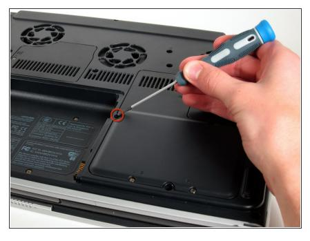
Remove the 8mm Philips screw located between the hard drive and the WiFi card.
