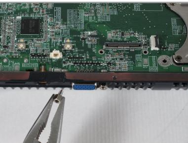
Using pliers, unscrew and remove the two bolts from both sides of the blue VGA connector.
