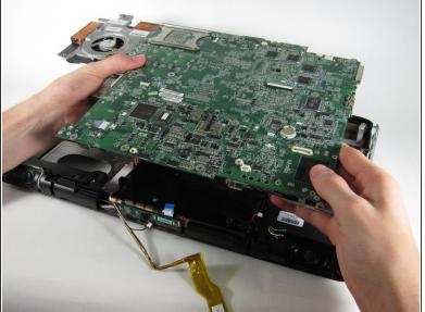
• Lift the motherboard up until it releases from the bottom casing and remove it from the laptop.
