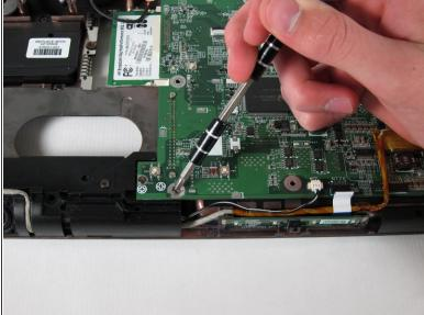
• Unscrew and remove the five 4mm Philips screws marked with the white Phillips screw icon.
