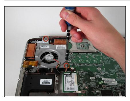
Unscrew and remove the two 8mm
