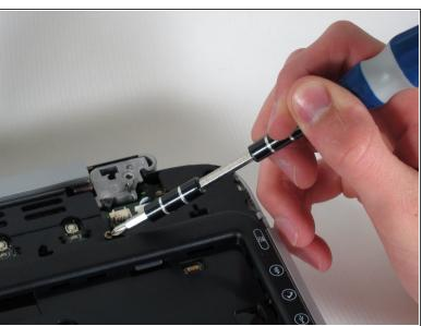
Unscrew the four 8mm Philips screws from the top cover.
