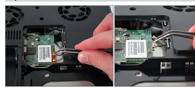
• Use <u>tweezers</u> to detach the grey and black cables connected to the green WiFi card.
