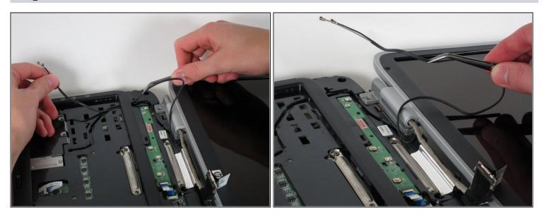
Using tweezers, pull the black cable towards the display and through the hole in the casing.
