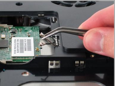
• Use tweezers to detach the grey and black cables connected to the green WiFi card.
