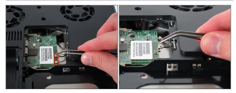
• Use <u>tweezers</u> to detach the grey and black cables connected to the green WiFi card.
