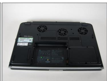
• Pull up on the battery to remove it.
