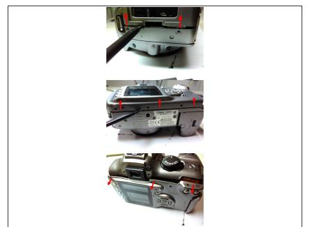
Use a plastic opening tool to help detaching the back casing from the camera's body.
