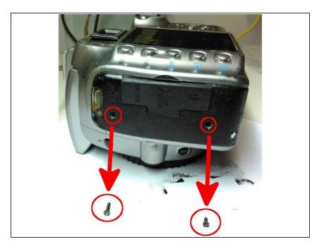
Remove the black screws from the camera's left rubber covering - note it is a 5/16" screw at the top and a 3/16" screw at the bottom.
