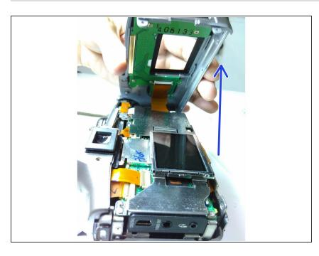
• Carefully lift the back casing from the camera's body from left to right.
