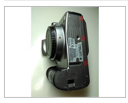
Remove the three 1/8" philips screws from the bottom of the back casing
