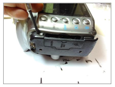
Aided by a screwdriver or plastic opening tool, remove the rubber coating from the left side of the camera.
