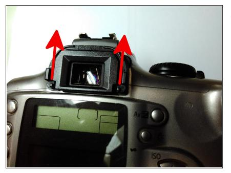
Remove the eyecup by gently pushing it upwards, so it doesn't block us in the final step of pulling the back casing from the camera's body.
