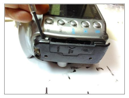
Aided by a screwdriver or plastic opening tool, remove the rubber coating from the left side of the camera.
