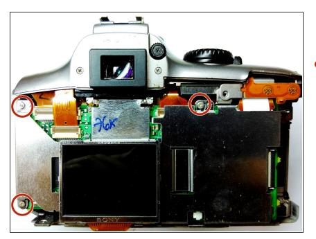
Remove the three 1/8" philips screws holding the LCD chassis to the camera's body.
