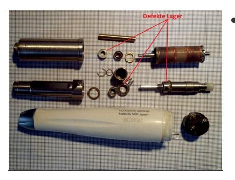
The picture shows the items. In the handpiece are the motor housing with the top right anchor.
