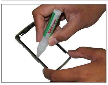
Apply super glue around the edge of the housing where the class will sit.
