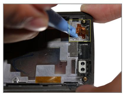
In the top right corner of the housing use a pry tool to disconnect the touch screen digitizer connector from the housing.
