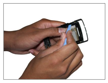
Use a safe prying tool and pry around the perimeter until the screen is separated from the housing.
