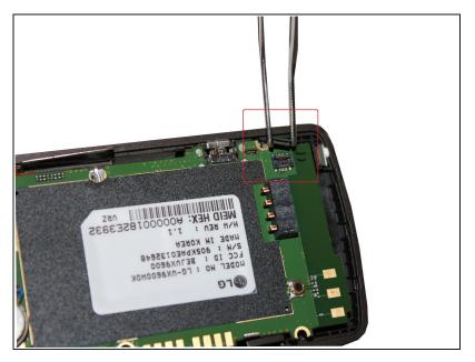
In the bottom right corner of the logic board, disconnect the button connector with tweezers or a prying tool.
