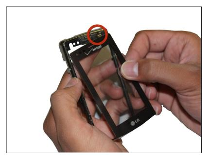
Put the ribbon cable through the hold and place your new touch screen inside the housing.
