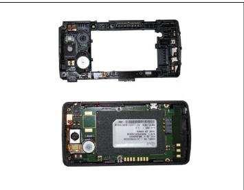
• Insert a safe prying tool between the slot between the front screen housing and the battery housing to remove the battery housing.
