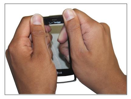
Push the housing and the glass together. Wait 5-10 minutes for glue to dry.
