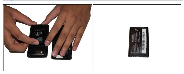
Simply insert your finger in between the slot and the battery and push down and up to remove the battery.
