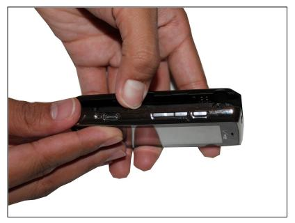
On the right hand side of the LG Versa there is a latch to open up the back of the cell phone. Push the latch up and lift off the back of the phone exposing the battery.
