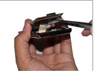
• The LCD screen is connected to the bottom of the logic board. Once you lift the logic board use tweezers or a safe prying tool to disconnect the ribbon wire from the LCD screen to the logic board.
