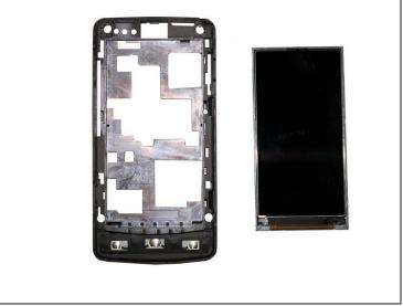
• Simply lift the LCD screen from the logic board housing to remove the LCD screen.
