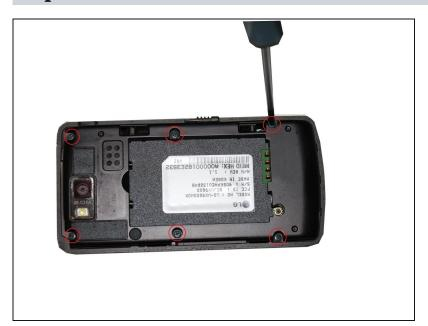
Six Phillips screws holding down the battery housing (Circled in the picture).
