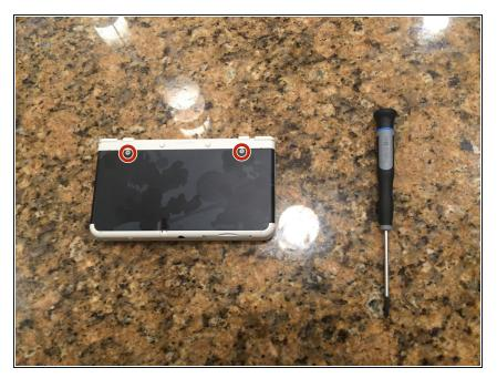
Use a size #0 phillips-head screwdriver to loosen the screws from the back cover plate. The screws are attached to the cover, so they will not come out completely.
