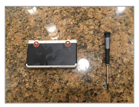
Attach the new back cover plate and tighten the two #0 phillips-head screws.
