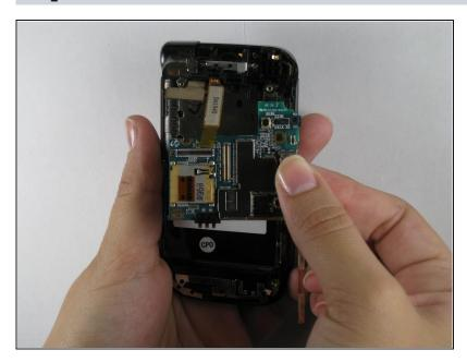
• Remove the logic board.
