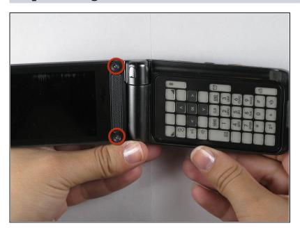
Use a Phillips #00 screwdriver to remove the two 4 mm screws on screen.
