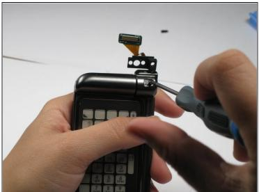
• Remove the 3.41 mm screw out from underneath plastic cover.
