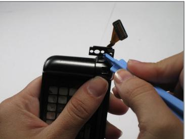
• Pop out the top half of the hinge with the plastic opening tool. This will release the hinge cover for removal.
