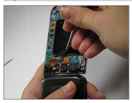
• Remove ribbon connector next to camera using tweezers.
