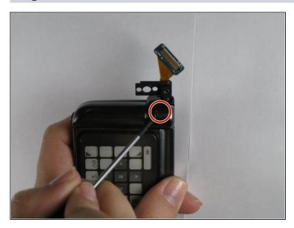
• Remove the plastic panel cover from the hinge.
