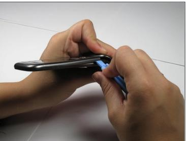
• Use the opening tool to remove the front outside casing.
