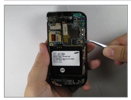
• Disconnect the connecting cord using tweezers.
