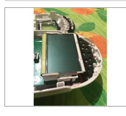
The LCD is held on by a pair of small plastic lugs, one each side. Release these one at a time, while
