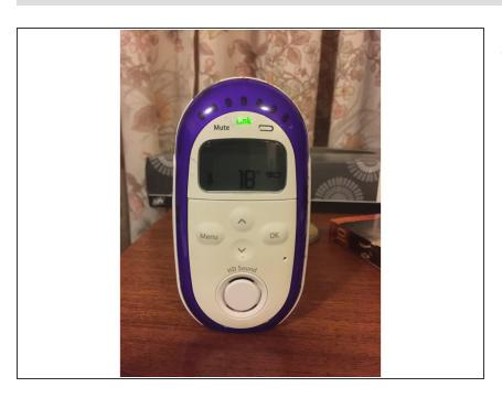
Unclip the battery cover, and remove the batteries (they're a tight fit - the purple ribbon should help though)
