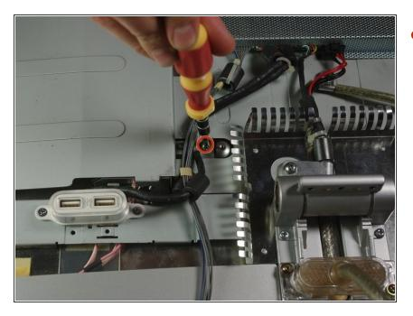
Unscrew the USB cable routing screw (8 x 2.72mm) using the PH 2 screwdriver.
