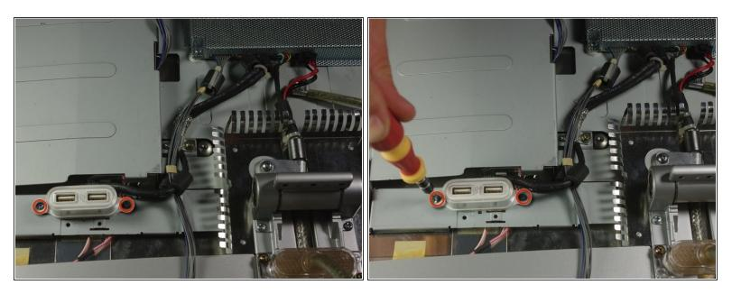
● Using the PH 2 screwdriver, unscrew the two screws (4.85 x 2.94mm) on the USB ports.
