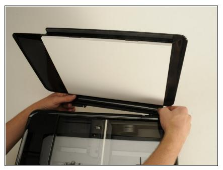
Remove the flap for the scanner.
