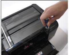
Remove the three screws from the top of the printer with a T-9 screwdriver as shown.
