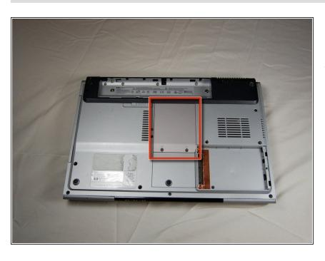
Locate RAM access door on the bottom side of the laptop.
