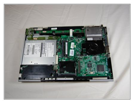
With the back cover removed, locate the CD drive.
