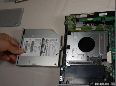
• With a firm grip on the CD drive's outer casing, slide it away from the laptop.
