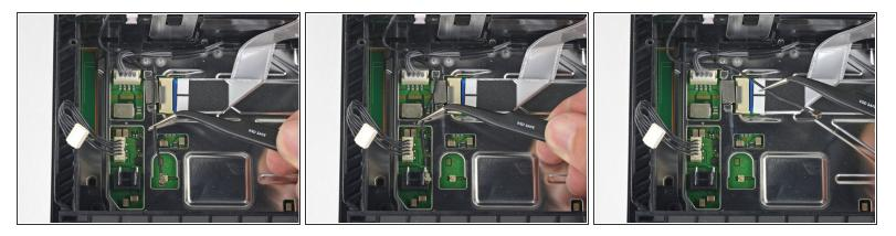
Use a pair of tweezers or your fingers to grab the antenna cable and move it out from the cable guides.
