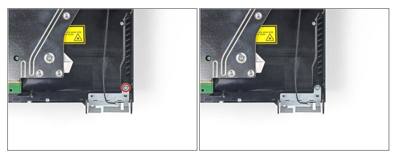
Remove the 9.7 mm Torx security screw securing the antenna.
