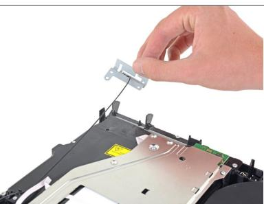
Remove the Wi-Fi antenna.
