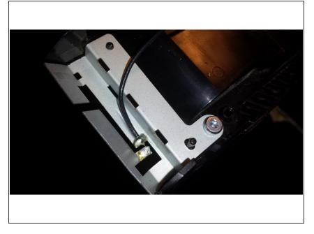
As you can see there are 2 solder points . the wire must run through the first point to the second point. But when the system fell it broke that connection and Antenna got bent. If at factory the solder points were not correct it will cause the same lag issue with controller and WiFi.
