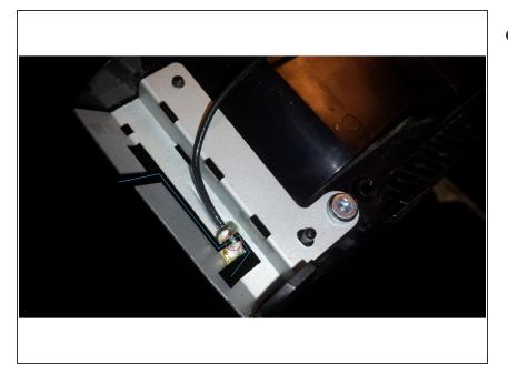
This is the easy part. Remove the antenna. Move the wire inbetween the two solder points so it is connecting to the second point. Once there take your soldering Iron and heat up the solder and drag it over the wire to make the connection.
