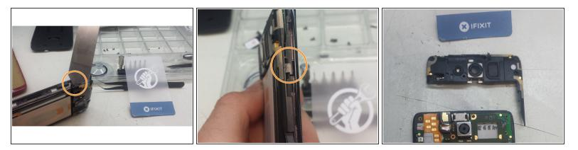
• With the iSesamo tool, or a prying tool, unclip the tabs on the left and right side of the phone.
