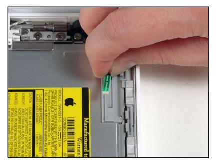
• Lift the Bluetooth antenna board from the front edge of the optical drive.
