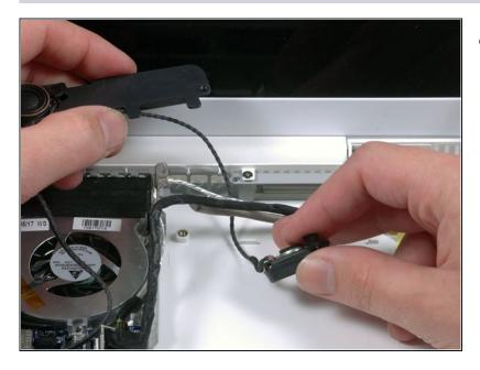
Thread the subwoofer and right speaker beneath the display data and microphone cables.
