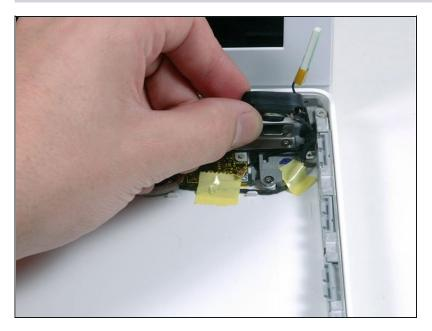
• Lift the right speaker out of its housing in the lower case.
