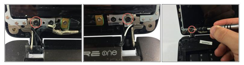
Remove the screws located on the four corners of the screen.
