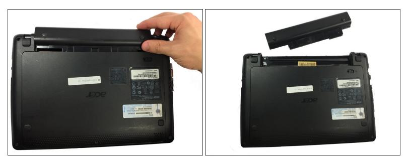
• If necessary, remove the old battery and replace it with a new one.
