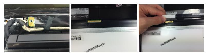
• On the bottom left of the screen there is a cord attached. Remove the tape that is attached to the screen.
