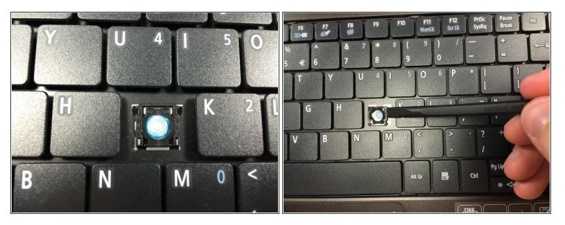
Use a spudger to pry the upper portion on both sides of the mechanism until it pops off from the key socket.
