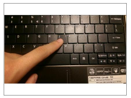
Place the key on top of the empty key space and press it down firmly until the key locks in place.
