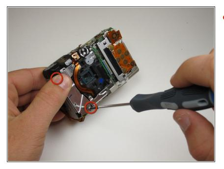
Flip the camera over again so that the rear is showing and remove the two .065 inch screws holding the flash unit in place. They should be on the left side.
