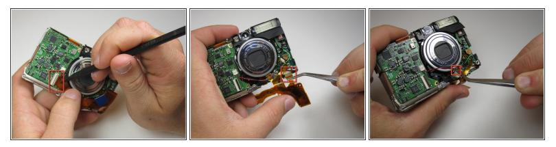
• One by one, detach the three ribbon cables from their ports.
