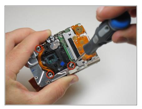
Next, remove the three .12 inch screws that hold the lens assembly to the camera.
