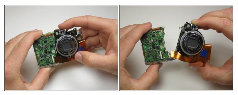
• Finally, pull the lens assembly away from the camera frame. Make sure that none of the ribbon cables are tangled up.
