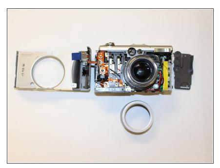
Next remove the front panel and right side panels (the left side is part of the front).
