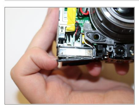
After that you can lift up the capacitor housing by using your finger nail, or other small object, to lift it up around the edges.
