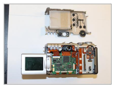
Once the screws have been removed, Remove the back panel.
