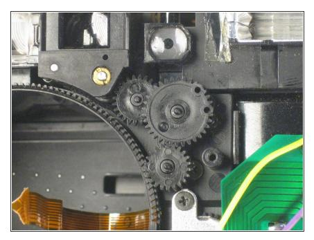
Remove the three gears under the panel you removed in the last step and the lens motor should be able to be removed.
