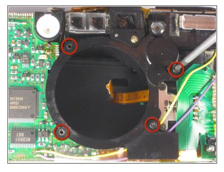
Remove the four screws holding on the front panel surrounding the lens.
