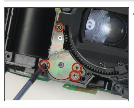
Unscrew the four screws on the back of this piece to the lower-left corner of the lens.
