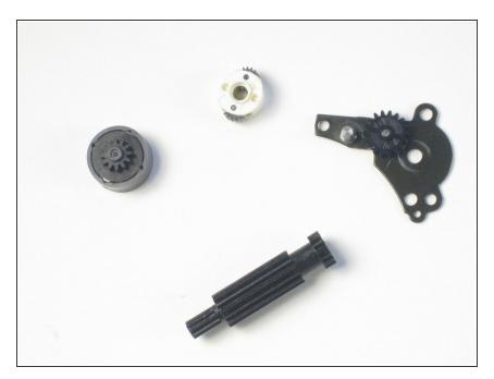
Removing the lens motor cover, you should be left with these four pieces.
