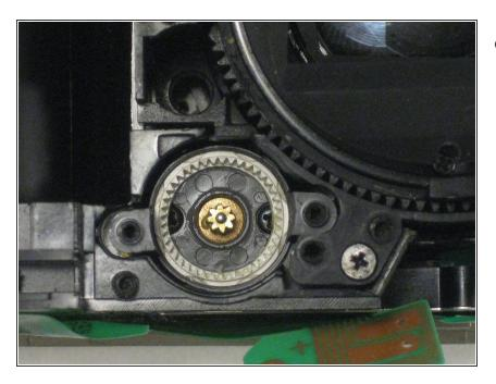
Located underneath these four pieces is the lens motor.
