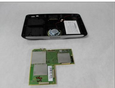
Now remove the motherboard out of the device. You will have two separate pieces.
