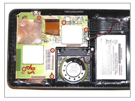
Using your T-4 Torx Screwdriver, unscrew six 1.58 mm T-4 Torx screws from the motherboard.
