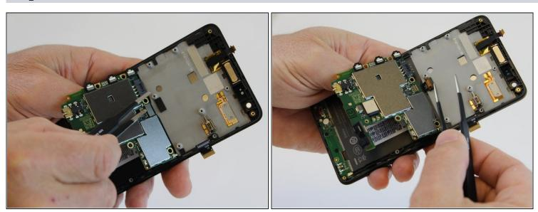
• Using one prong of the tweezers, lift and pry back the metal clip positioned over the front proximity sensor ribbon connector.
