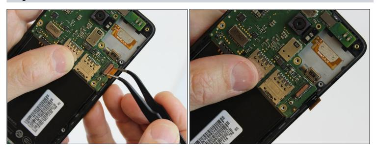
• Using one prong of the <u>tweezers</u>, pry back the brown clip located on top of the LCD ribbon connector.
