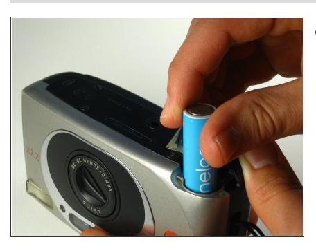
From here, simply insert a new CR123A Lithium battery.
