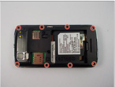
Using a T4 Torx driver, remove the eight 4 mm back panel screws.
