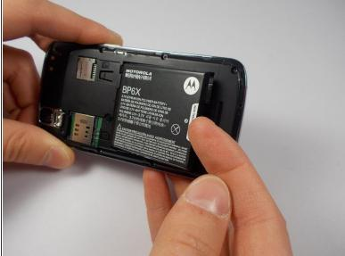
Remove the battery using the thumb tab.
