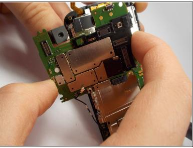
To remove the motherboard, pull it to the side. The camera that is connected to the motherboard does not pull straight up and out from its holder.
