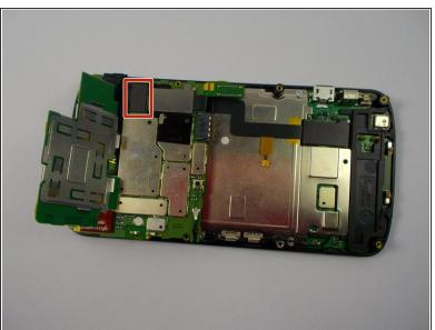
Gently lift the SD & SIM card board (PCB) as shown.
