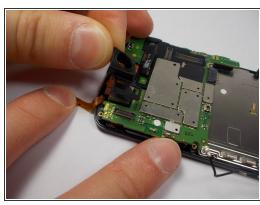
Remove the camera's rubber seal by pulling it off. It is not connected to anything.
