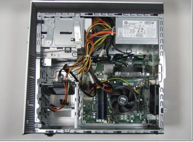
Next, remove the side panel by sliding it towards the back of the desktop and pulling up, as shown.
