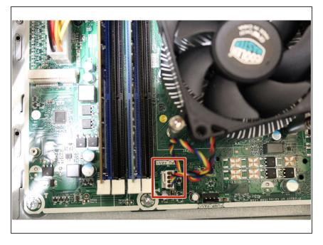
Carefully pull up and disconnect the fan's power cable.
