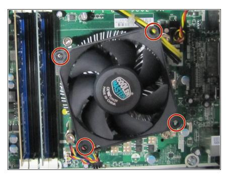
Remove the four 120mm Phillips #000 head, 5 mm screws holding the fan.
