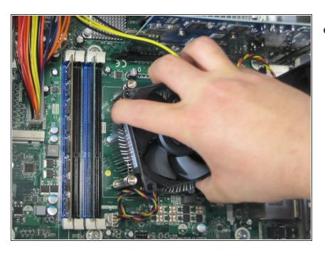
Remove the fan by pulling up carefully.
