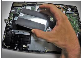
Once disconnected from the tape and the connector is free, lift the Hard Drive unit from the rest of the device by grasping each side with thumb and index or middle finger. To reassemble your device, follow these instructions in reverse order.
