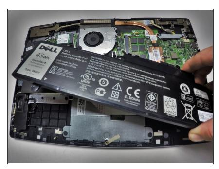
Gently remove the battery from the rest of the device.
